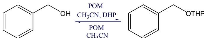
Scheme 1. Tetrahydropyranylation-depyranylation of benzyl alcohol in the presence of (\text{NH}_4)_8[\text{CeW}_{10}\text{O}_{36}]\cdot 20\text{H}_2\text{O} .
