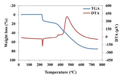
Fig. 1. Thermal behavior of 1.
