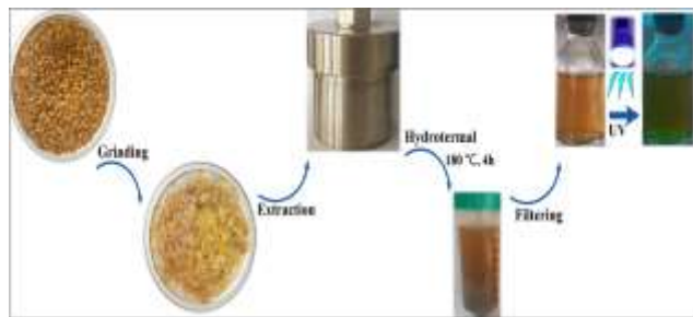
Fig. 1. The synthesis schematic of CQD from Trigonella foenum-graecum L seeds extract.
